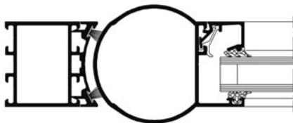
Anti-pince-doigts sur ouvrant arrondi Finger-pinch protection on rounded opening frame
